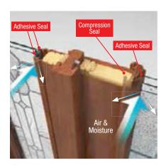
Cip-lite frame (shown right) features a compression seal against weather on the outside of the door and an adhesive seal against weather on the outside of the glass. Flush-glazed glass (shown left) is built directly into the door without a Lip-lite frame, featuring a high-performance adhesive weather seal inside and out.
