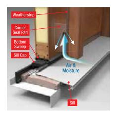
Corner seal pads (inswing only) complete the seal between the sill cap, bottom sweep and weatherstrip to help block potential pathways where wind-driven moisture can infiltrate the bottom corner of the door system.
