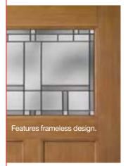
Glass built directly into the door during the manufacturing process eliminates the need for a lite frame and provides a high-performance weather seal. Flush-glazed glass features clean lines and eliminates the need for screw plugs. It also offers up to a 16% increase in visible glass area compared to conventional lite frames.
